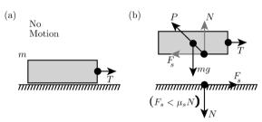
A cord is attached to a block of weight W = mg and the tension,  $\underline{T}$ , in the cord is such that the block remains at rest (diagram (a)). Diagram (b) is the corresponding separated body diagram.  $\underline{P}$  is the force exerted on the block by the surface. N and  $F_{\circ}$  are the components of  $\underline{P}$ , normal to and parallel to the surface.  $\underline{F}_s$  is called the force of static friction. From Newton's 2nd law,
